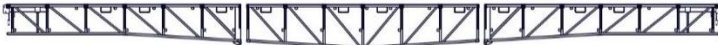
Bridge assembly 60'-0" (18,30 m), with two (2) bridges of 20'-0" (6,10 m) and a central bridge 20'-0" (6,10 m)
