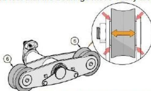
Figure 7-Roller and bearing movement
