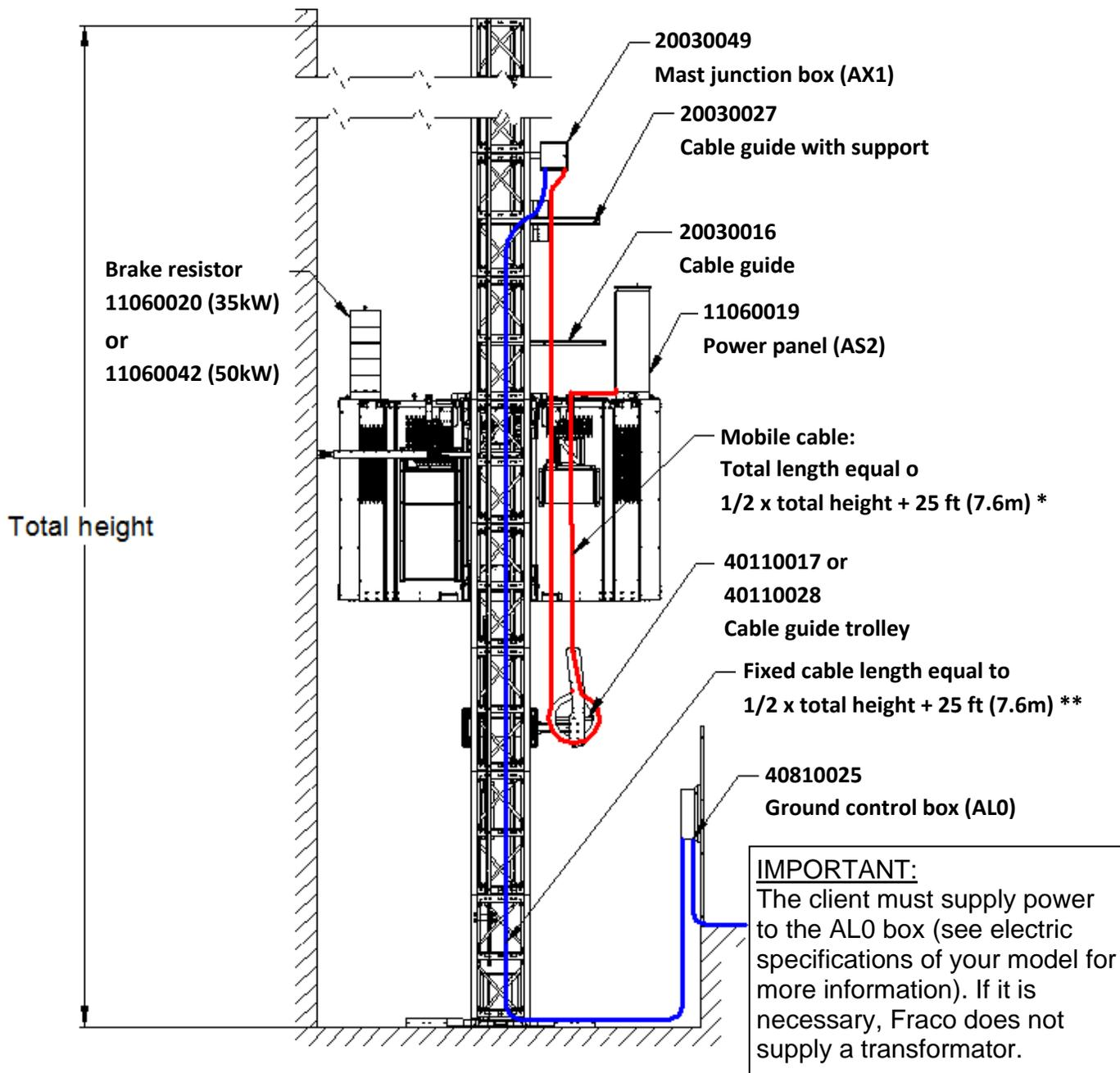
\* Mobile cable must be type **DRAKA INDUSTRIITE, 4 strands** (Strands dimension depend on model). **Any other type of cable must be approved by Fraco to be used.**
