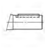
High speed shaft end
